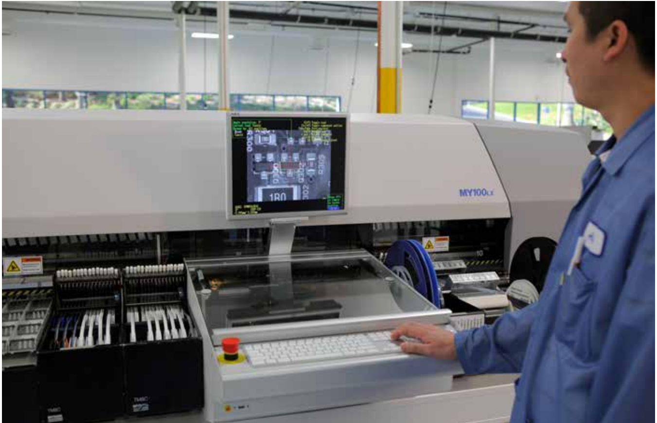
SAI's SMT lines utilize equipment optimized for fast changeover, which reduces costs for high mix production. Equipment is set up to run completely by machine from solder paste application through placement and reflow to decrease time and save costs.
