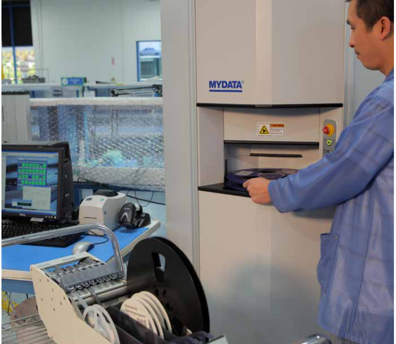
Automated processes eliminate the potential for defects. SAI uses component towers for point-of-use material stocking. The tower provides an ESD and humidity-controlled environment for component storage. Parts are scanned via a barcode that corresponds with the job number to decrease defects, as well.
