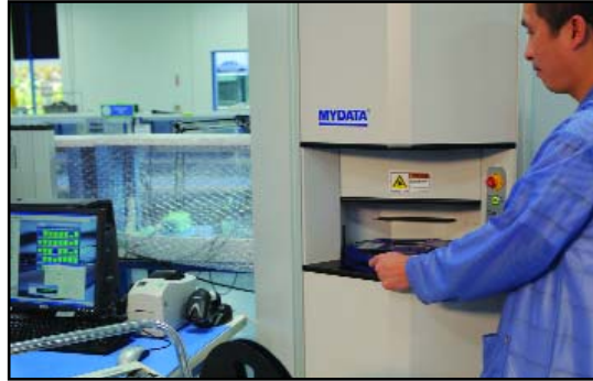
Humidity-controlled component towers are linked to the MRP system and support line-side stocking.
