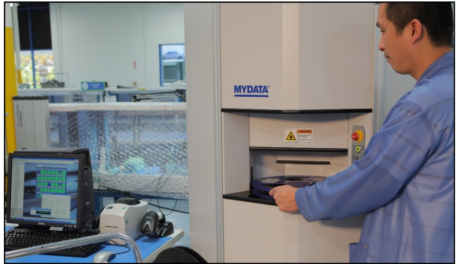
Component towers minimize handling by putting components at point-of-use.
